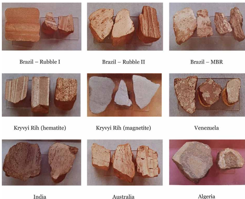
Figure 2. Iron ores (the photographs were created from atlas of ores [3] by the authors of this chapter).
