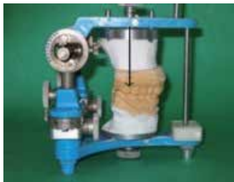
Fig. 8. Vertically movable upper mounting ring.
