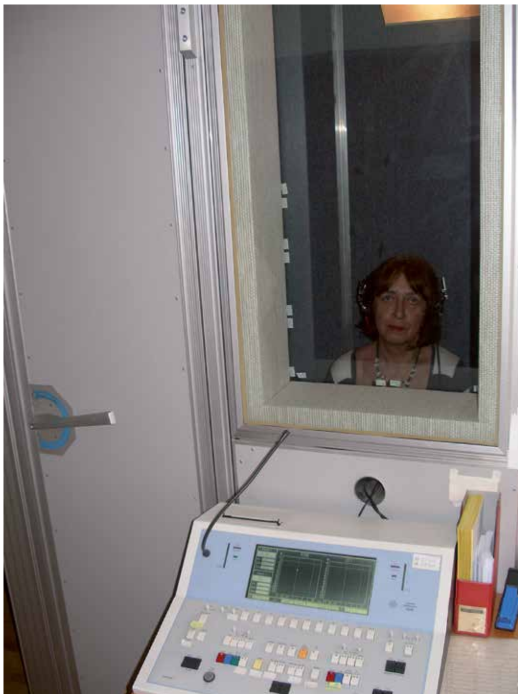
Fig. 1. Clinical Audiometer AC 40, Interacustics, Denmark used for measurement of thresholds of audibility and specification of tinnitus.
