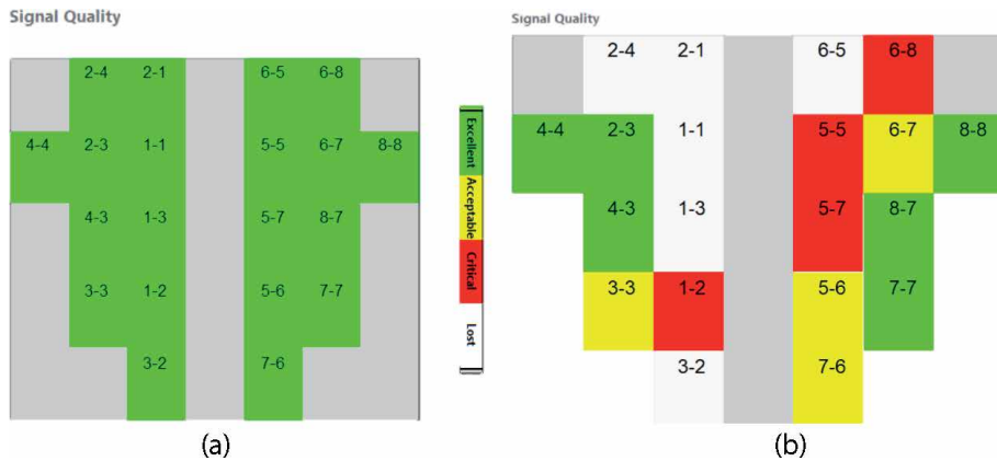
Figure 3. Visual representation of optode settings. The perfect setting is illustrated in (a) meanwhile the faulty optode settings are shown in (b). The color bar on the right side represents the signal quality class.
