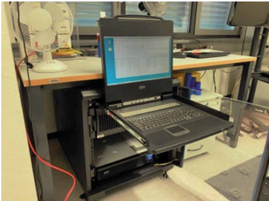
Figure 14. Real-time controller with MQTT server.
