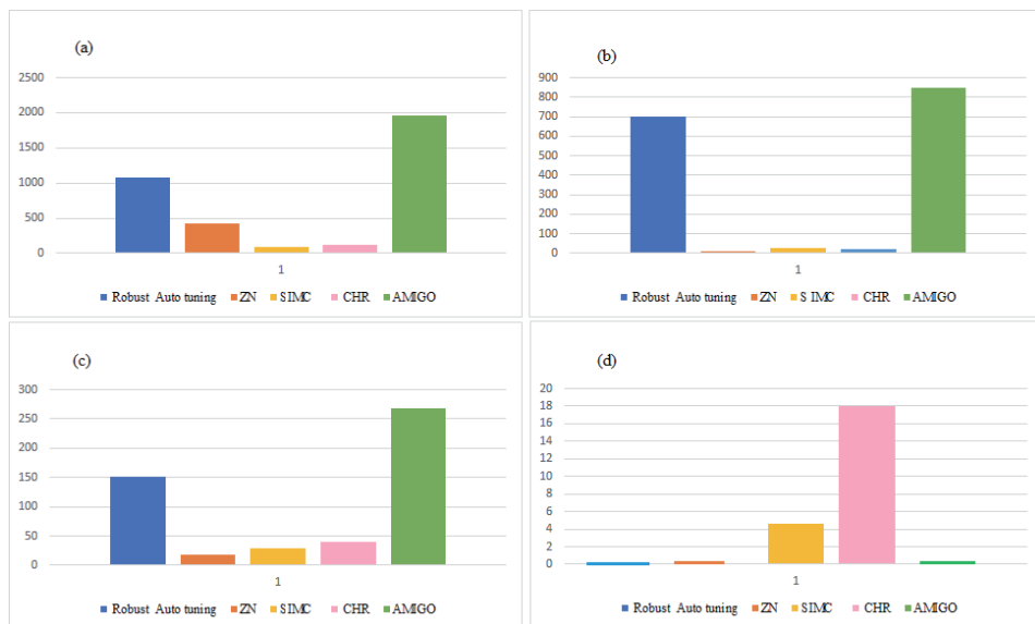
Figure 14. Comparative improvement time response specifications between tuning methods based OBT with respect to tuning lonely, (a)improvement td ratio, (b) improvement tr ratio, (c) improvement ts ratio, (d) improvement overshoot ratio.
