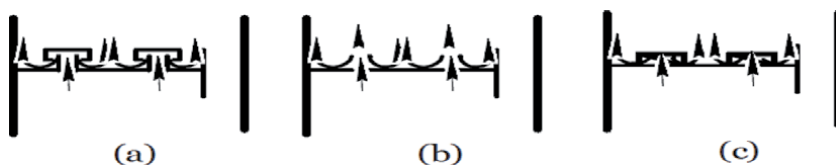
Figure 9. The types of plate in the column: (a) cap, (b) grid, (C) valve.
