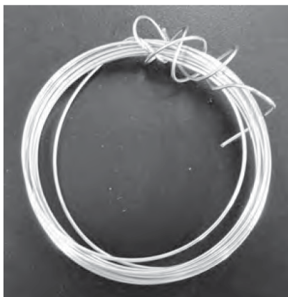
Figure 10. An inexpensive stainless wire as electrodes of electrophoresis tank. This wire is 1.2 mm in diameter.
