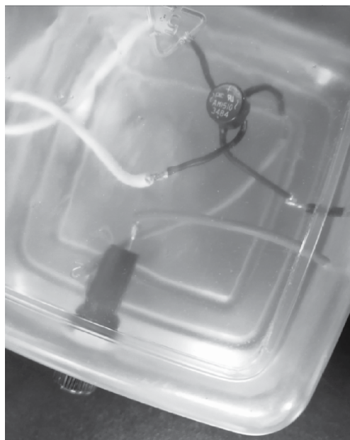
Figure 14. A close view of the DIY power supply (Figure 13). An inexpensive Graetz bridge (AM1510) is used in the supply.
