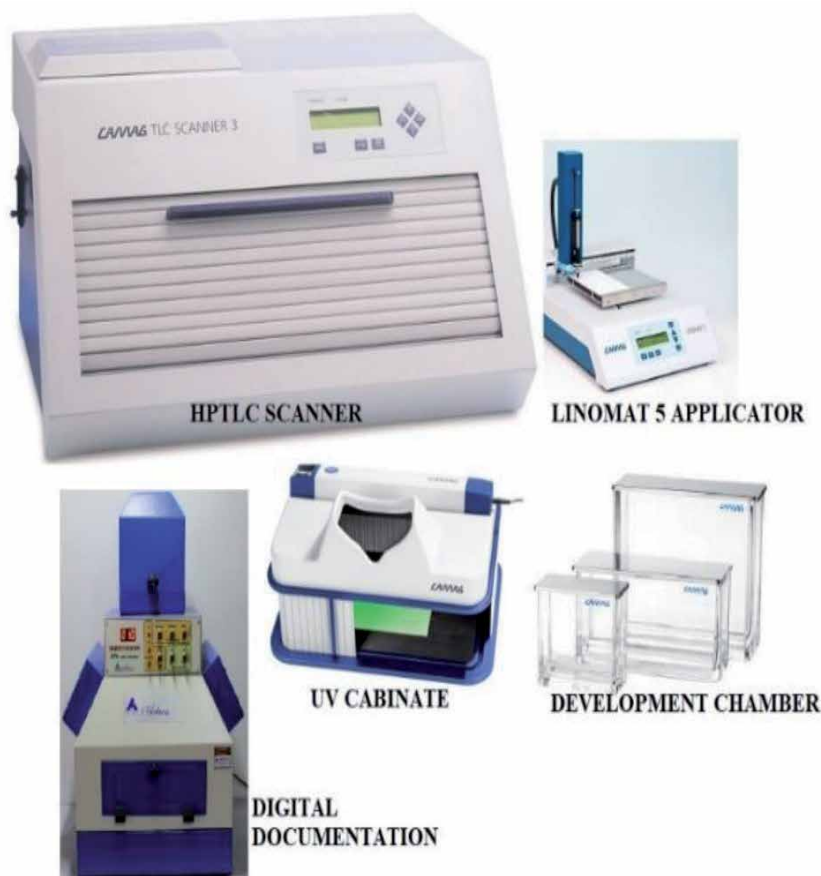
Figure 5. Diagram showing components of HPTLC.
