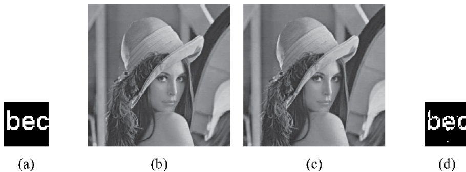
Figure 3. (a) Original watermark image. (b) Watermarked Lena, PSNR = 41.9914 dB. (c) Attacked watermarked Lena with JPEG-40 attack, PSNR = 34.9652 dB. (d) Extracted watermark, NCC = 0.9253 .
