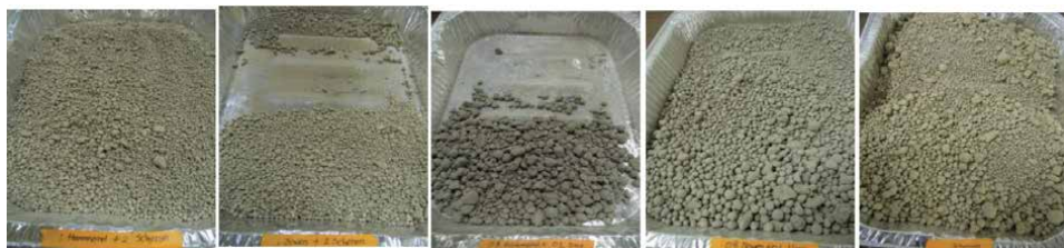
Figure 2. The five (5) types of CFA beads produced from the three (3) CFA samples (from left to right: 1 CFA3 + 2 CFA1; 1 CFA2 + 2 CFA1; 4 CFA3 + 1 Lime; 4 CFA2 + 1 Lime; and CFA1. Note: the numbers of 1, 2, and 4 are referred to mass ratios).
