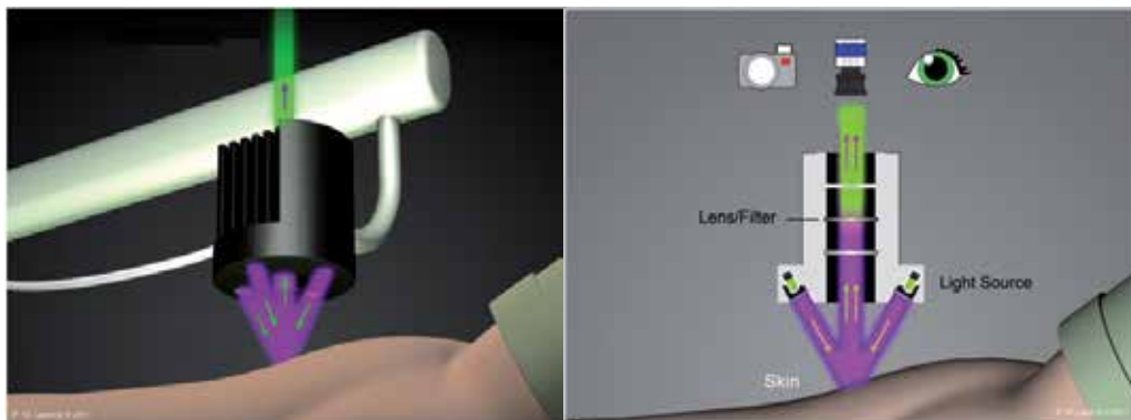
Fig. 2. Possible configuration of an image system. The light interacts with the skin and is re-emitted. The emission can be magnified by lens and the colors selected by optical filters. The visualization can be performed by a camera or naked eye.
