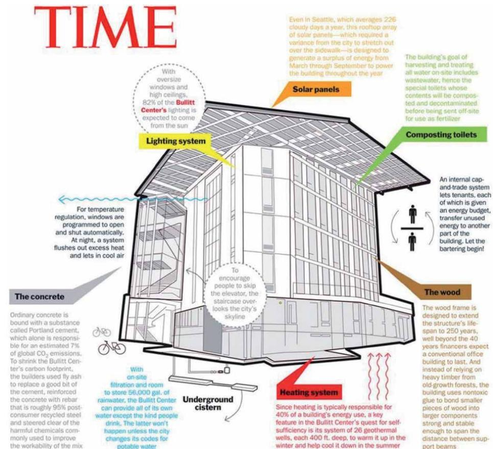
**Figure 4.** Seattle's net-zero energy building (Bullitt Center) [17].
