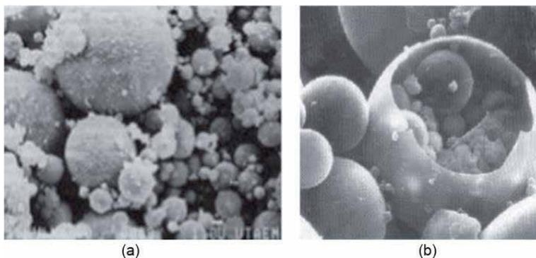
**Figure 1.** Scanning electron microscope of FA: (a) cenosphere and (b) plerosphere particles [7].
