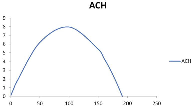
**Figure 15.** Effect of solar chimney size on the air change per hour of the lecture room.
