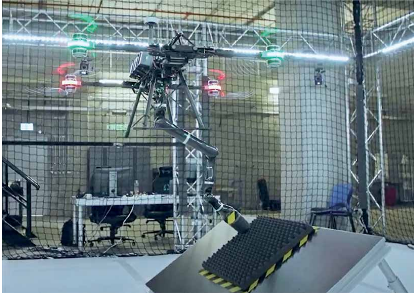
Figure 19. Surface ultra-sound scanning utilizing aerial manipulation.
