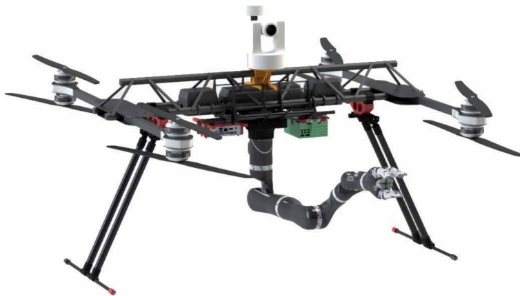
Figure 18. Aerial manipulation system with PTZ-camera.
