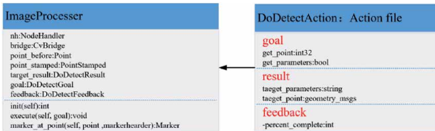
Figure 21. Image processing node UML design.
