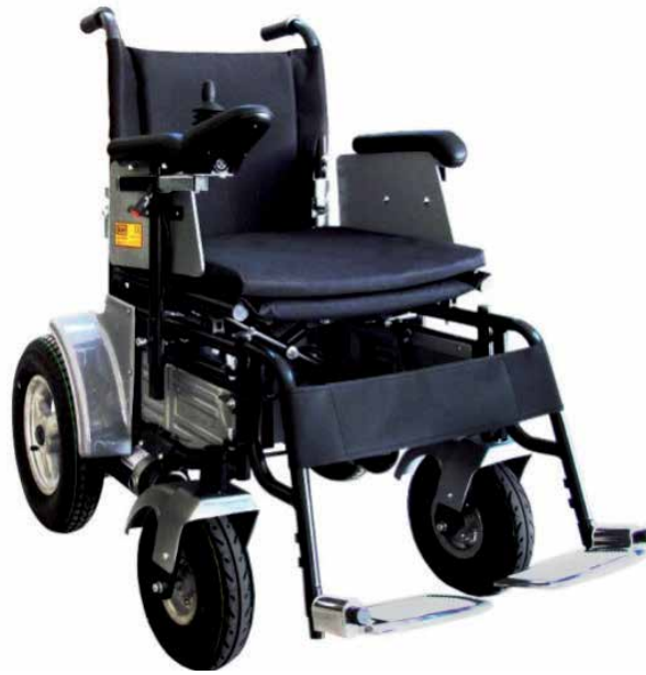
Figure 1. Conventional electric wheelchair used as a base system for conversion.
