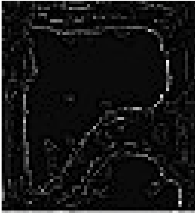
Fig. 6. The result of the Laplacian filter applied to the example image of figure 3b.
