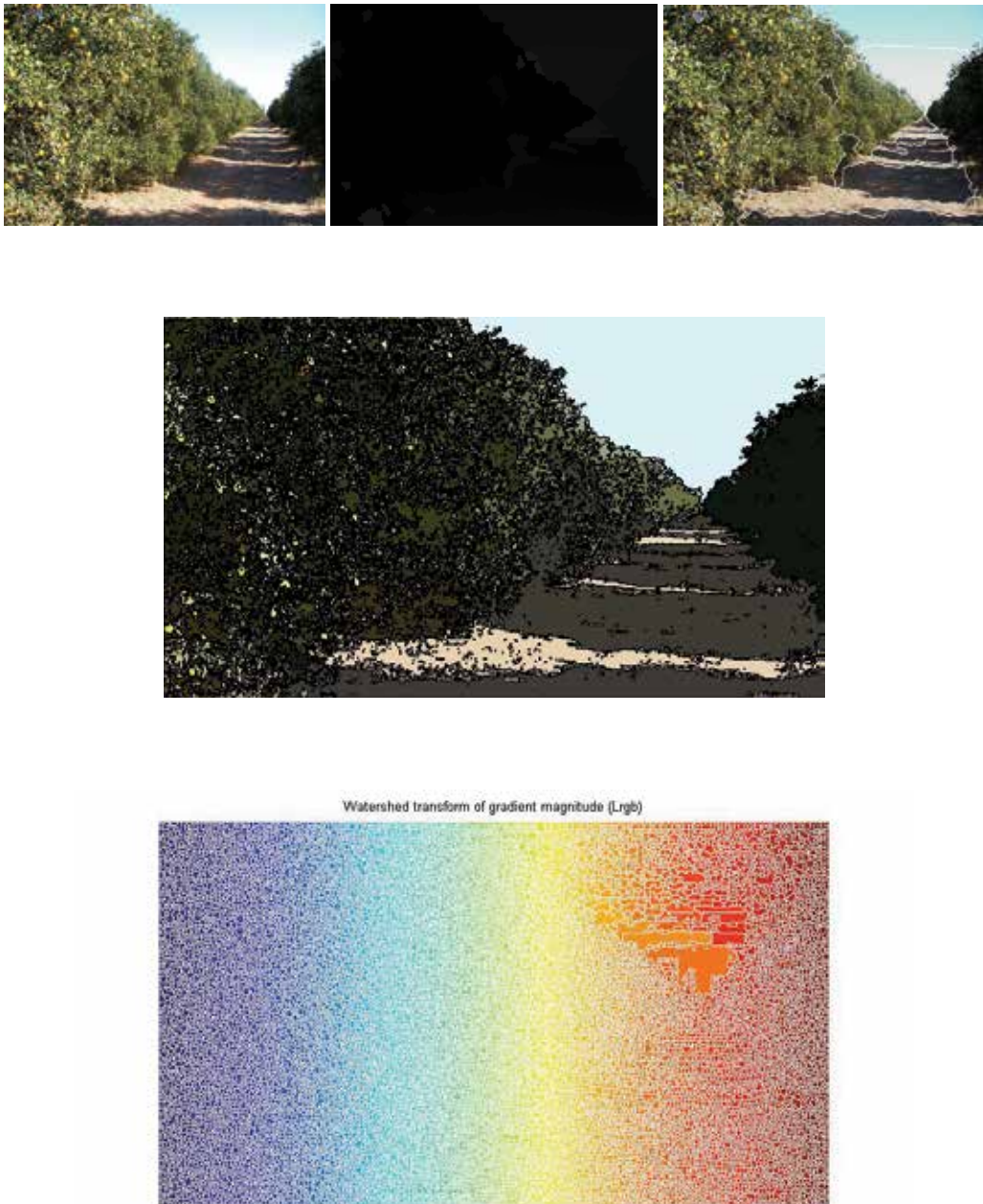
Fig. 9. JSEG segmentation and watershed transform of gradient magnitude in flood fill class-map for scene 4.
