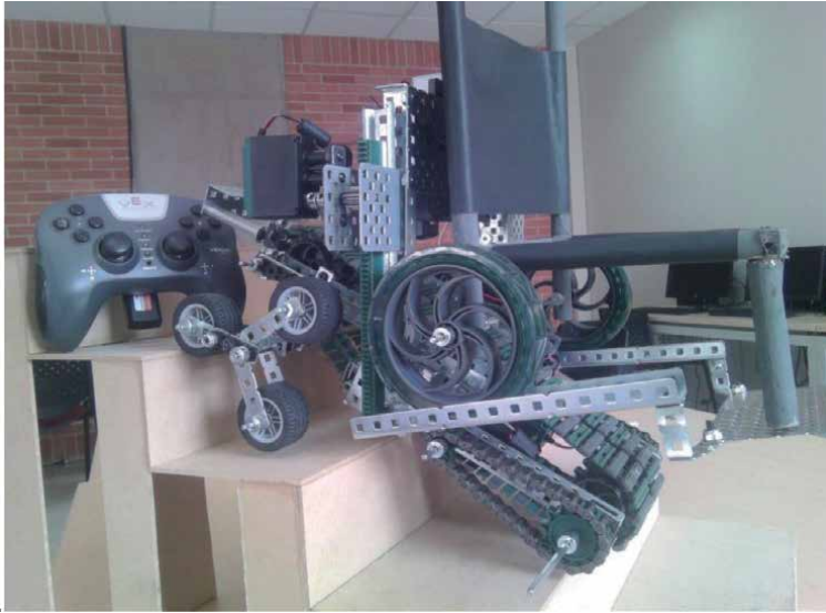
Figure 7. Up and down movement of the wheelchair. Source: Author.
