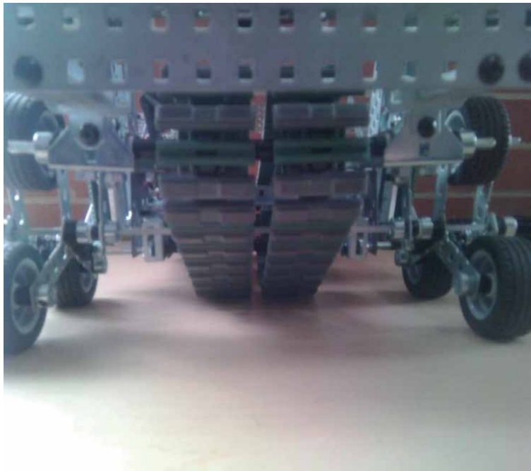
Figure 6. Chair of wheels with design of caterpillars.
