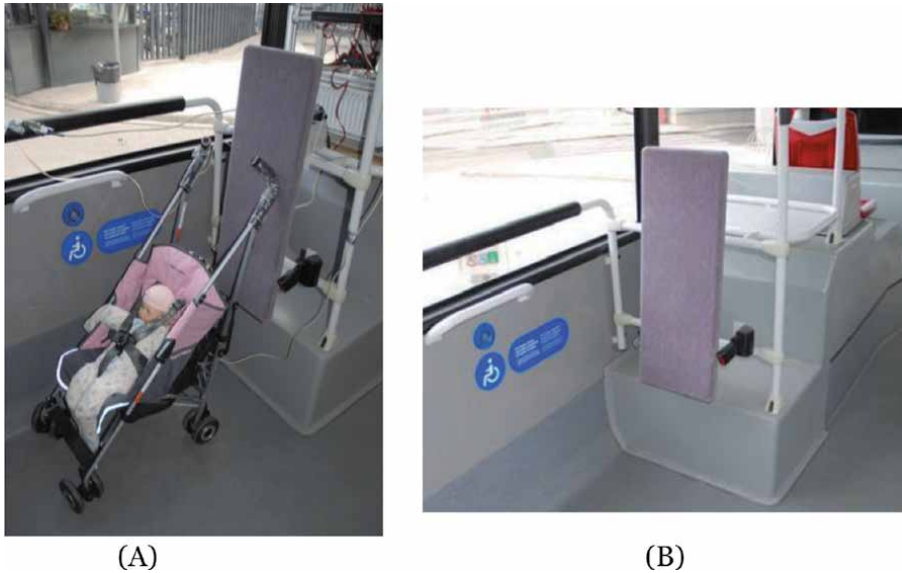
Figure 8. Most adequate position of unfolded ChC for traveling in M3 vehicles: (A) with space occupied by ChC; (B) with space unoccupied by ChC (source: [14]).
