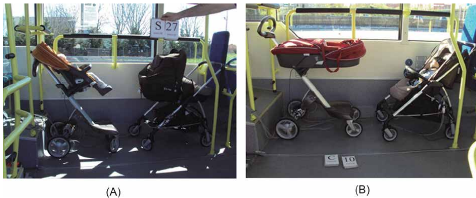
Figure 6. Provision of ChC deployed during experimental open circuit trials: (A) unfolded rearwards facing Model A carriage and forwards facing Model C carriage; (B) unfolded rearwards facing Model B carriage and forwards facing Model C carriage (source: [14])
