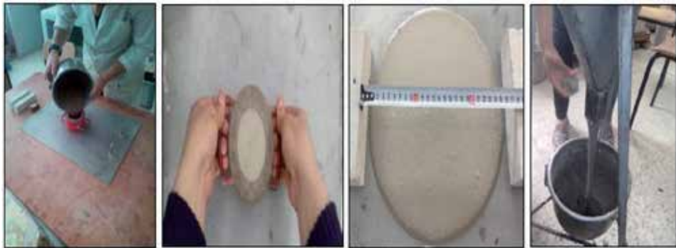
Figure 7. Fluidity measurement test of FSC.
