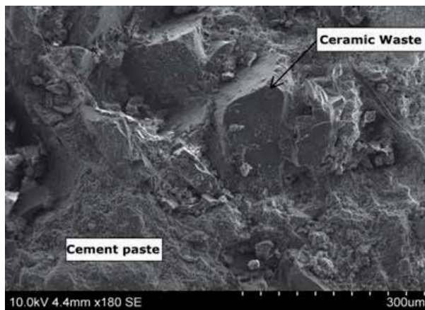
Figure 12. SEM image showing the good adhesion of CW with cement matrix in FSC.
