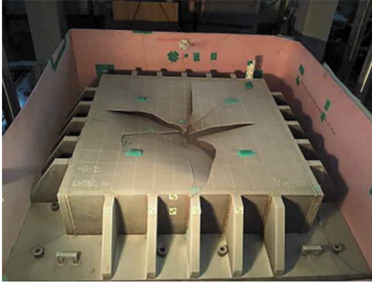
Figure 3. Brittle fracture of a steel stiffened-panel under dropped-object impact at -60°C [44].
