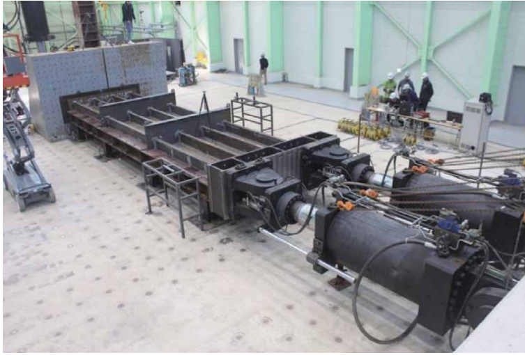
Figure 4. The axial-compressive collapse test set-up of a full-scale steel stiffened plate structure [1, 7, 8].
