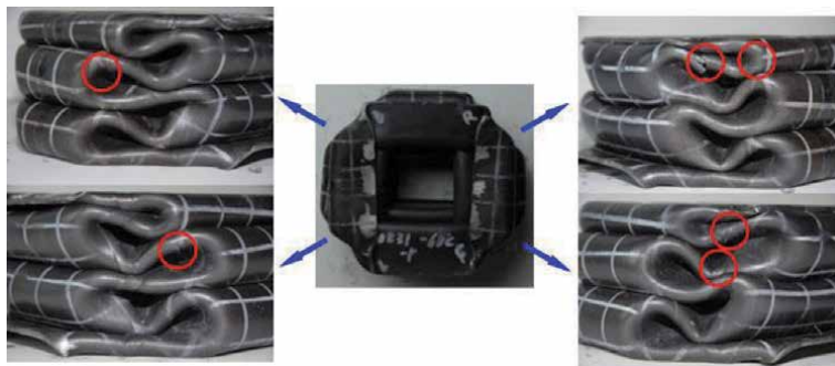
Figure 2. Ductile fracture of a square tube under quasi-static crushing loads at -60^{\circ}\text{C} [42].
