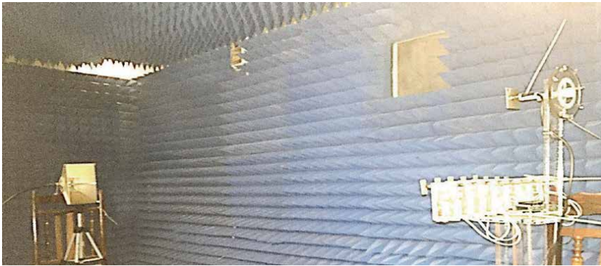
Figure 31. Array antenna measurement in anechoic chamber.
