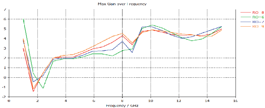
Figure 15. Gain diagram with effect of the antenna radius.
