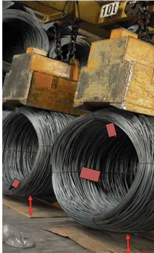
Figure 10. Steel coils with RFID tags lifted by the overhead crane, magnetic field emission in the environment.
