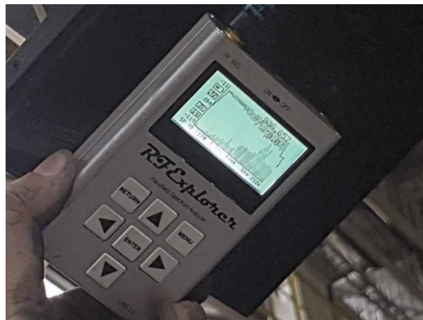
Figure 11. Spectrum analyzer measuring the frequencies radiated in the environment during the RFID reading tests with the electromagnetic overhead crane connected.
