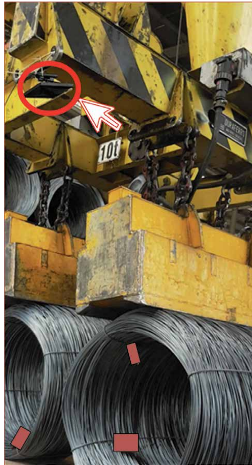
Figure 9. RFID antenna installed on the overhead crane for the RFID tag reading tests.
