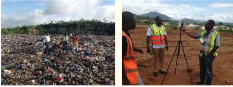
Figure 7. The A-S500 portable gas instrument with sensors being mounted on the Nsumia landfill and a control site for GHG measurements.
