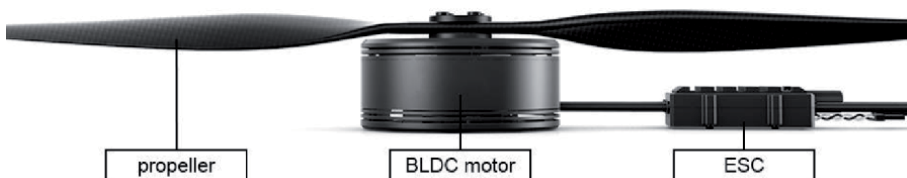
Figure 5. Multirotor UAV electric propulsion unit.
