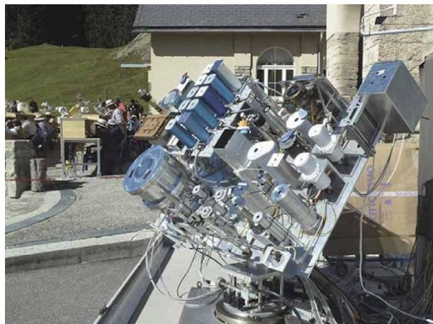
**Figure 16.** World standard group (WSG) of absolute cavity pyrhemometers at WRC PMOD in Davos Switzerland [28].
