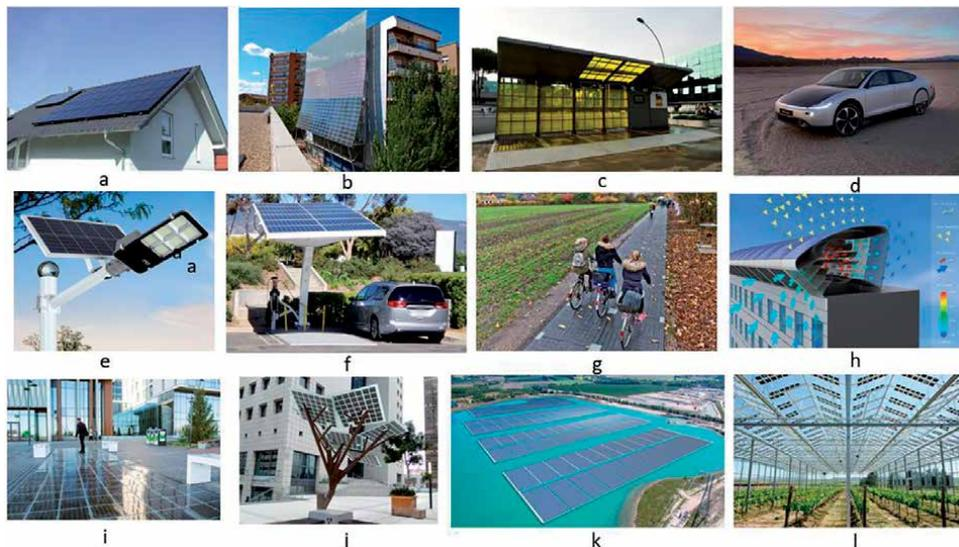
**Figure 9.** Various examples of novel applications of photovoltaic technology are as follows: (a) BAPV [20], (b) BIPV [21], (c) LSC PV [22], (d) VIPV [23], (e) solar street lights [24], (f) PV charging stations [25], (g) PV bike path [26], (h) PV windrail [27], (i) solar-powered pavement [28], (j) PV tree [29], (k) floating PV systems [30], and (l) agri-voltaic system [31].
