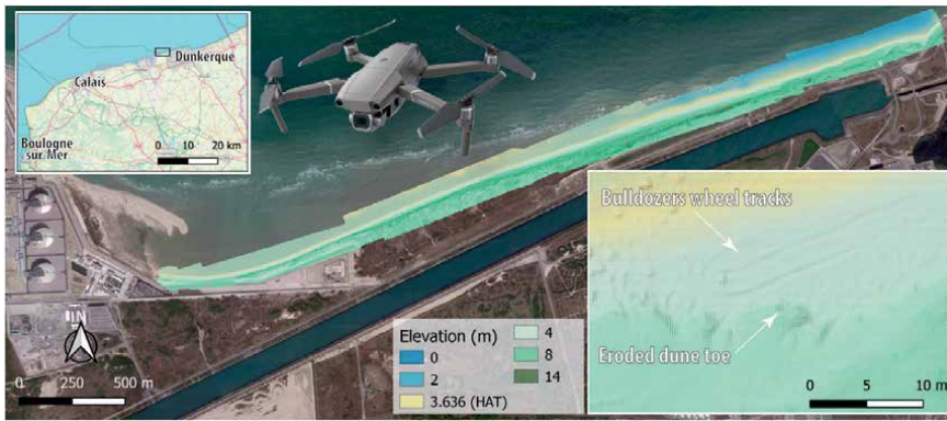
Figure 5. Example of a very high resolution DSM computed from photogrammetric survey carried out with a DJI Mavic 2 Pro UAV on the harbor of Dunkirk coast, northern France.
