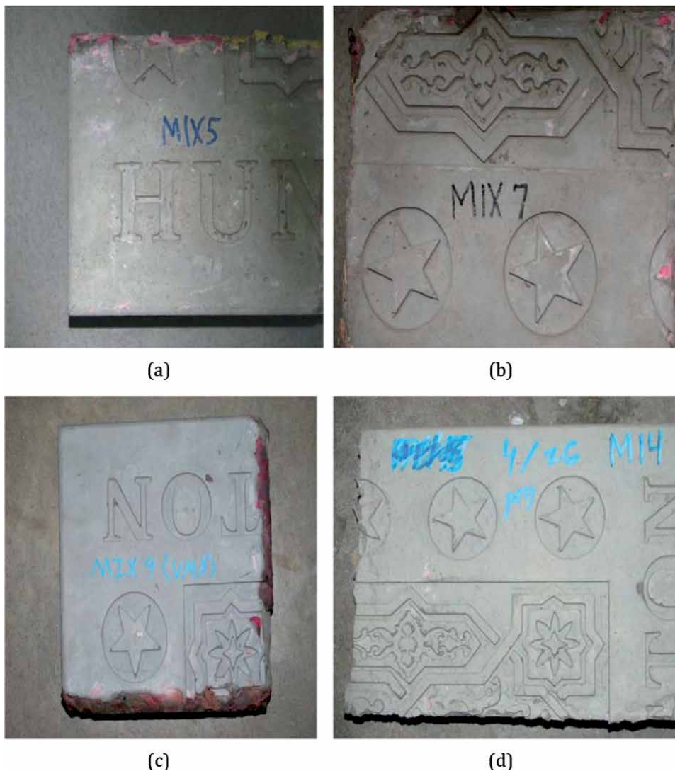
Figure 5. Smooth finishes of SCFRC samples made from different batches: (a) batch 5, (b) batch 7, (c) batch 9, (d) batch 14.
