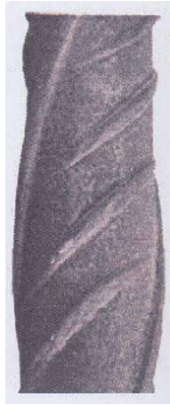
Figure 1. Typical cold twisted deformed (CTD) rebar, with lugs and protrusions on the surface and stresses beyond yield on the entire body, which replaced plain round bars starting the decade of the 1960's.
