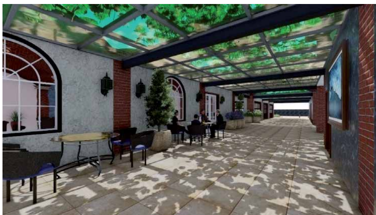
Figure 9. In buildings it is possible to have vines/creeper covered trellises which provides shading in summer, allows diffused sunlight. Source: Created by Nivedhitha Ravichandran.
