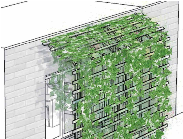
Figure 11. Window shaded by trellises with deciduous vines. Source: Co-author.
