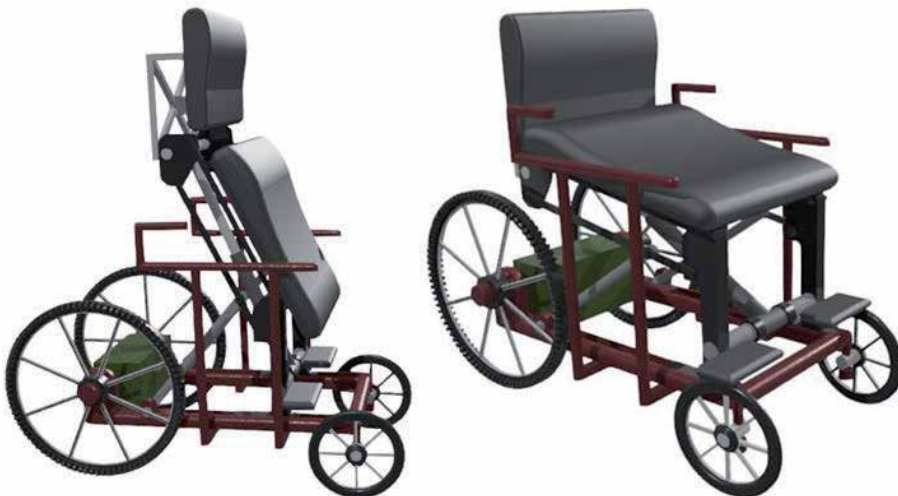
Figure 9. Linear actuator lift and recliner concept in seated and standing posture.
