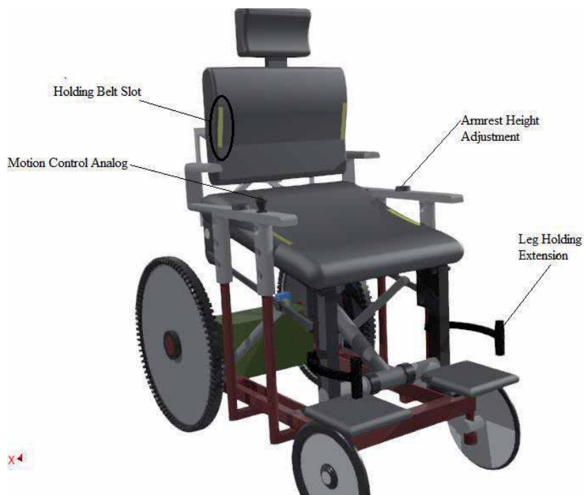
Figure 12. Support mechanisms including seatbelt, arm rest and leg holding extension.
