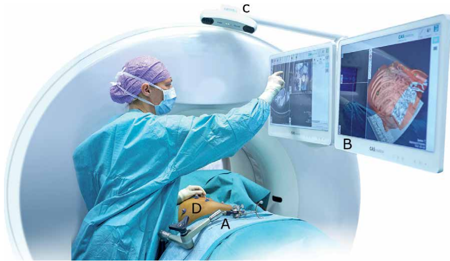
Figure 3. Setup for percutaneous needle insertion. Aiming device (A), touch monitors (B), optical tracking camera (C), patient markers (D).
