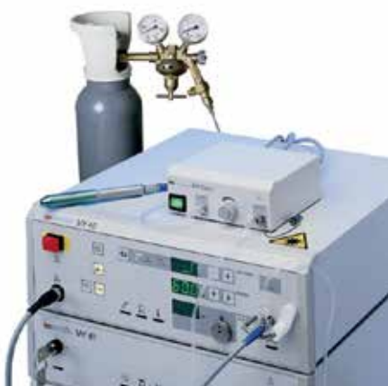
Fig. 1. Components of modern Laser equipment for the application on lung tissue (1318 nm wavelength, 40 W power output, beam quality, energy efficiency, high performance smoke evacuation system, 0.4 mm diameter of fibre, focusing handpiece, flexible quartz fibres /low water content/).
