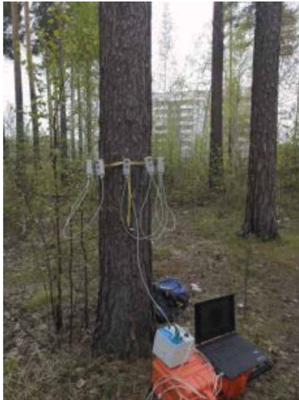
Figure 2. Arbotom® wood condition measurement.
