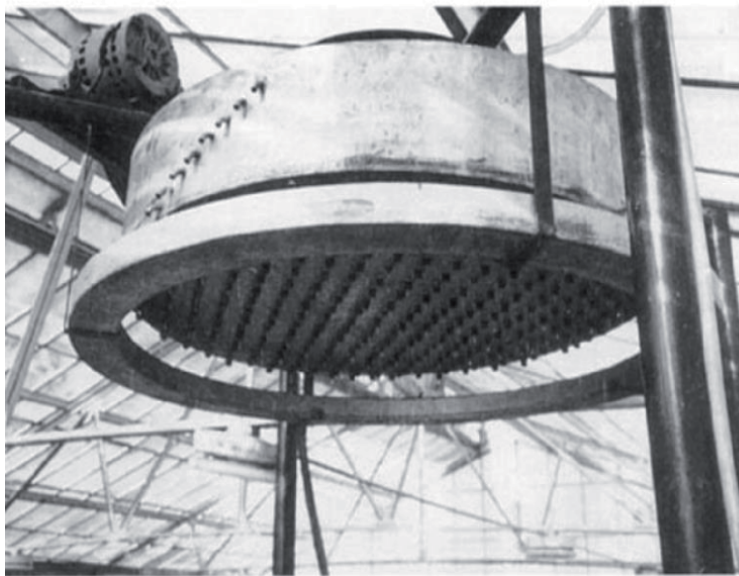
Figure 1. Drop formers simulator [11].
