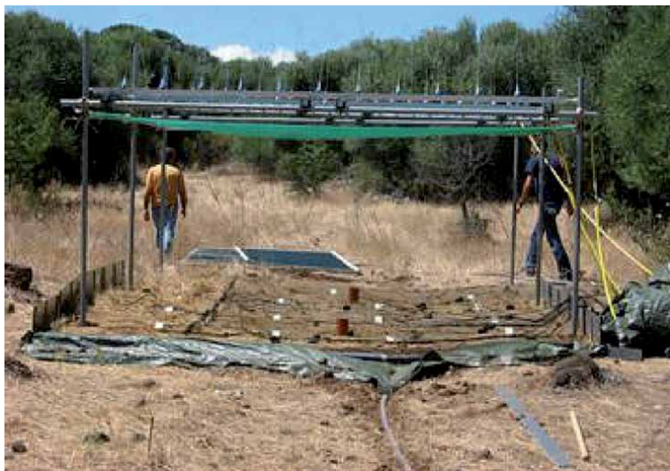
Figure 5. Outdoor rainfall simulator [13].
