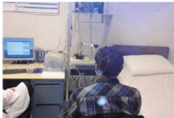
Figure 14. Experimental setup for a BMI based on a EEG demultiplexer.
