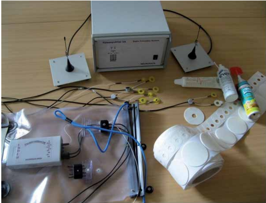
Fig. 1. The equipment for recording EMG signal in a water environment (Pánek et al., 2010).
