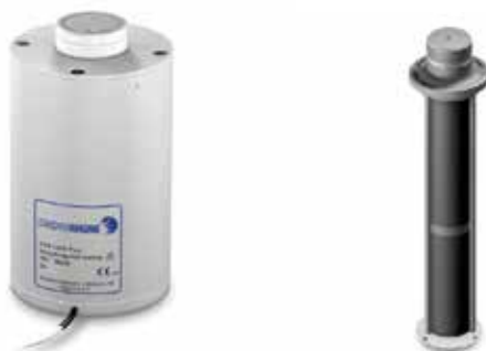
Fig. 5. A typical well-type ionization chamber, including a tool to performs tests of source positioning within 0.3 mm, timer accuracy, and consistency of source activity
