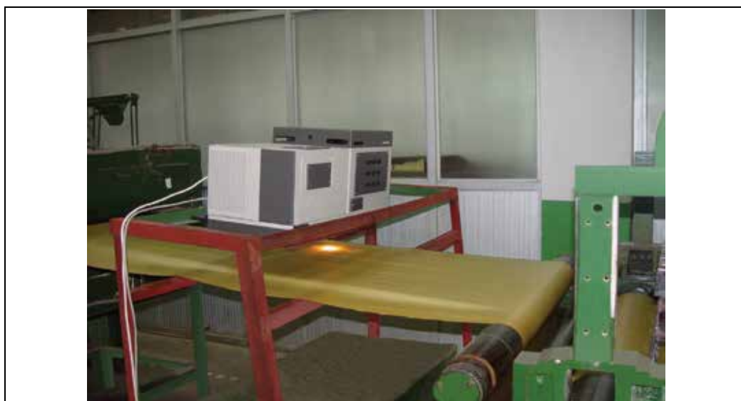
Fig. 7. Application of NIR for quality monitoring in the production of glass/phenolic prepreg cloth
