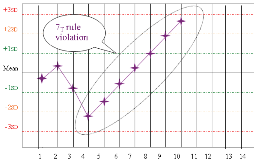
Fig. 11. Rule 7T – reject when seven control measurements trend in the same direction, either higher or lower.
