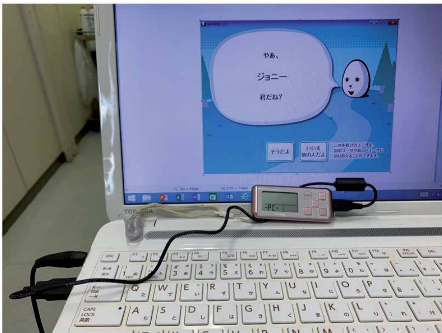
Figure 1. Citizen digital pedometer TW700, connected to a laptop computer. The pedometer was connected to a laptop computer through a USB cable to upload steps.
