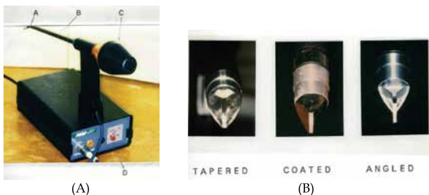
Fig. 10. (A) The IRK-151 infrared coagulator (a = tip; b = light-conducting quartz rod; c = reflector; d = timer). (B) Three kinds of artificial sapphire tips: (left) tapered, (middle) coated, and (right) angled. The coated tip has the same shape as the tapered tip, but the slanting surfaces are coated with nickel and tin dichloride. The angled tip has a 4-mm straight nose to prevent unnecessary ablation caused by direct contact of the slanting surface. When these sapphire tips are pressed into tissue, light energy is absorbed by the myocardium, which is then photocoagulated.
