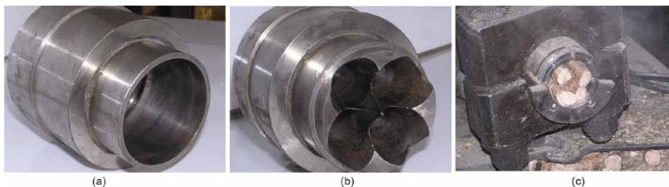
Figure 12. Briquetting press pelleting Hood [9]. (a) Briquetting hood, (b) hood with pelleting insert and (c) production of pellets.
