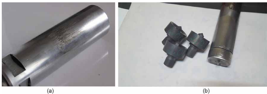
Figure 13. Press piston. (a) Wearing of a press instrument and (b) stacked piston.
