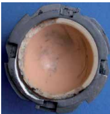
Fig. 10. Acetabular liner showing gross damage to the liner
