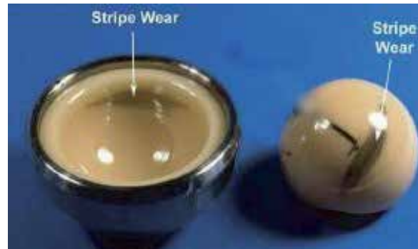
Fig. 11. A ceramic head and acetabular liner from a patient with “squeaking” hip with evidence of impingement and “stripe wear”.
