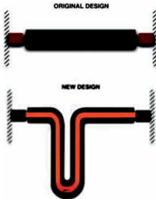
Figure 11. New and old design of refrigerating system.
