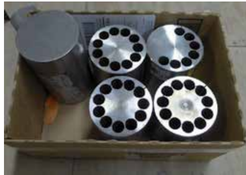
Figure 3. Axial tensile specimen extraction from bar stock.
