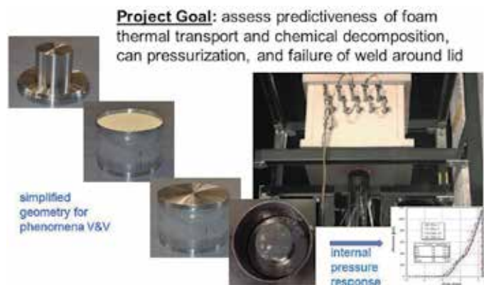
Figure 1. Thermal-chemical-mechanical validation experiments [2], including internal pressure response. The ‘can’ includes the cylindrical ‘sidewalls’ or ‘walls,’ as well as the top ‘lid’ and bottom ‘base.’
