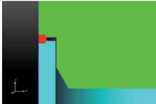
Figure 2. Close-up of modeled geometry where can top lid, sidewall, and internal foam meet. (Nominal geometry values are 0.03 in. weld depth, 0.0645 in. wall thickness, and 0.007 in. clearance between the lid and sidewall in the weld region.)
