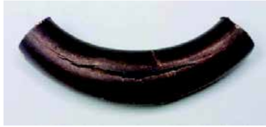
Figure 12. Macroscopic image cracked copper tube.
