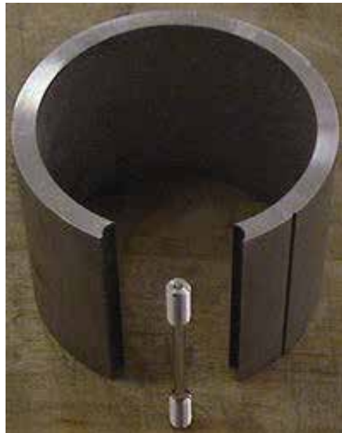
Figure 5. Axial tensile specimen extraction from wall material.
