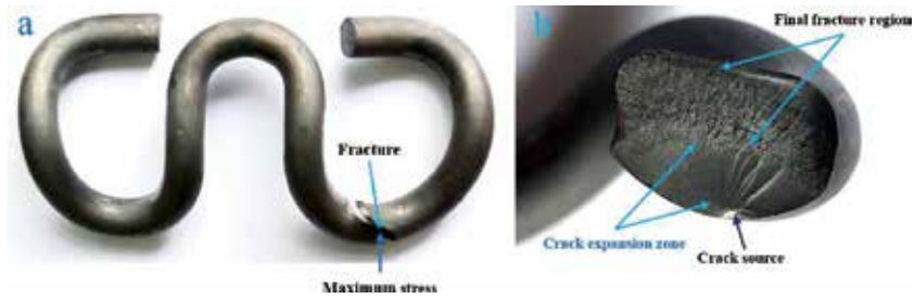
Figure 2. The macroscopic morphology of the premature fatigue fracture samples processed by the high-frequency-inducing heating.
