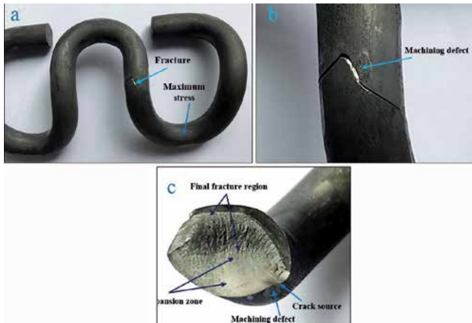
Figure 1. Macroscopic analysis of the premature fatigue fractured rail fastening clip caused by surface processing defects: (a) the overall morphology of the fractured clip, (b) the processing defects near the crack initiation region, and (c) the morphology of the fractured surface.
