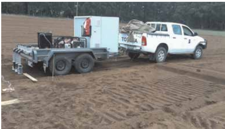
Figure 8. Prototype 4 by 2 kW microwave weed killer in a strawberry runner field at Toolangi, Victoria.
