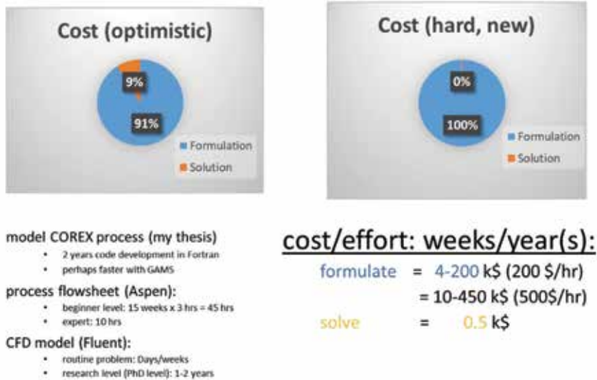
Figure 3. Overview of the cost of modeling. Problem formulation absorbs more than 90% of the cost for the development of mathematical models.
