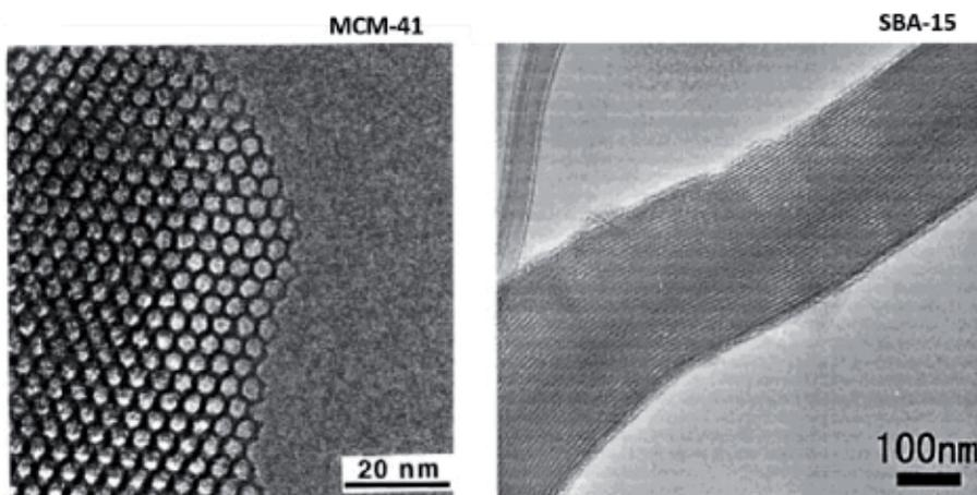
**Figure 2.** TEM micrographs for (a) MCM-41 (reproduced with permission from Ref. [24]) and (b) SBA-15 (reproduced with permission from Ref. [27]).
