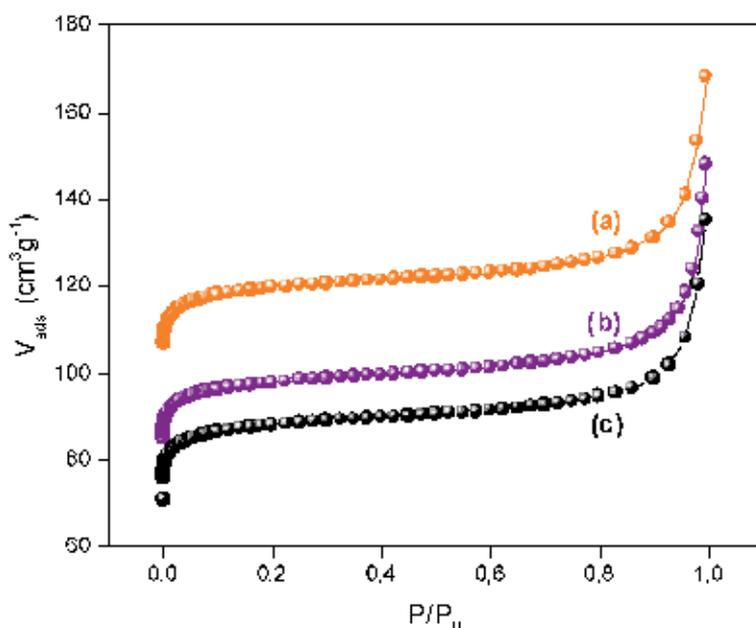
**Figure 18.** Adsorption/desorption isotherms of N<sub>2</sub> at -196°C obtained for (a) AC support, (b) Ru(4.3)-AC, and (c) Ru(8)-AC catalysts.
