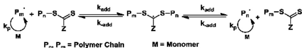
**Figure 4.** Addition-fragmentation equilibria during RAFT polymerization.
