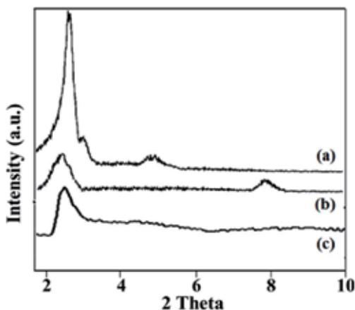
**Figure 5.** Low angle powder XRD of (A) MCM-48, (B) TPA-MCM-48 and (C) L-arg<sub>1</sub>/TPA-MCM-48.
