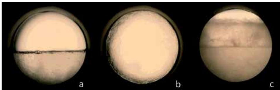
**Figure 1.** Phases observed with a high pressure cell: (a) heterogeneous gas/liquid, (b) phase transition and (c) homogeneous in supercritical state.
