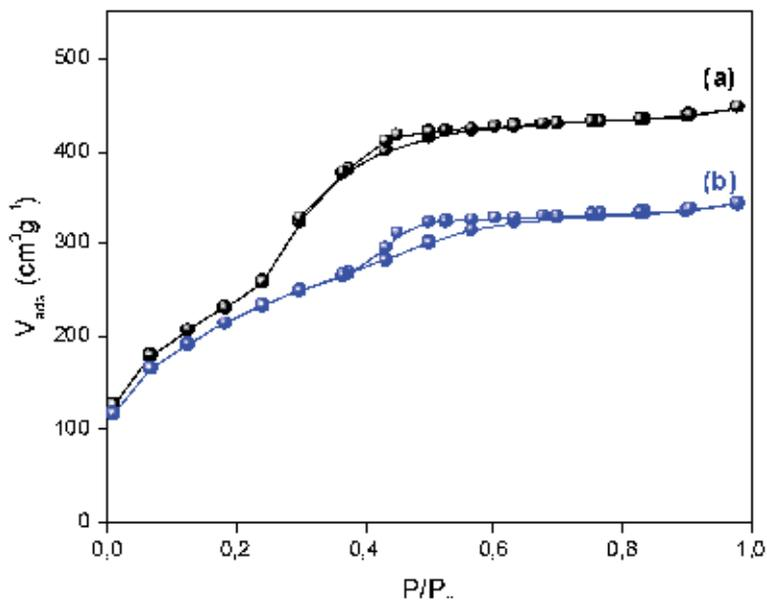
**Figure 15.** Adsorption/desorption isotherms of N<sub>2</sub> at -196°C obtained for samples (a) MCM-48 and (b) Ni-MCM-48.
