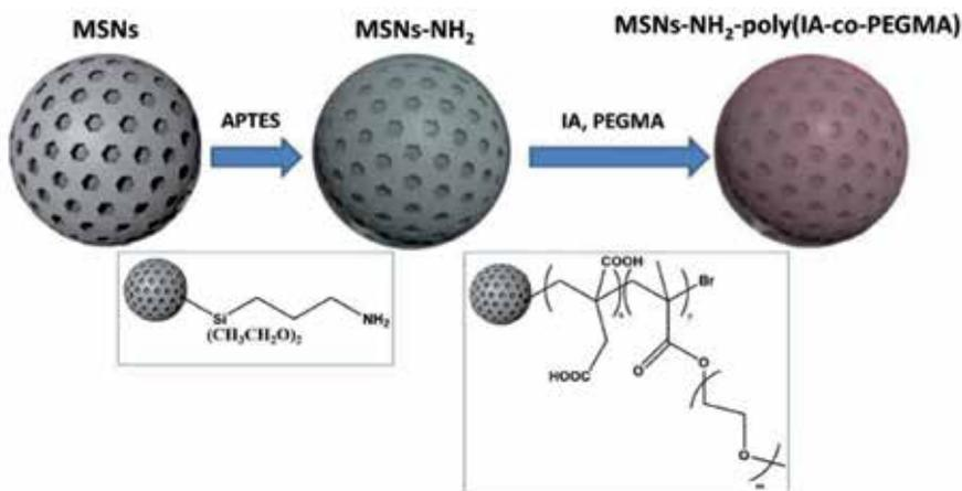
**Figure 9.** Synthesis route of MSNs-NH<sub>2</sub>-poly(IA-co-PEGMA) via a catalyst free ATRP (reproduced with permission from Ref. [35]).
