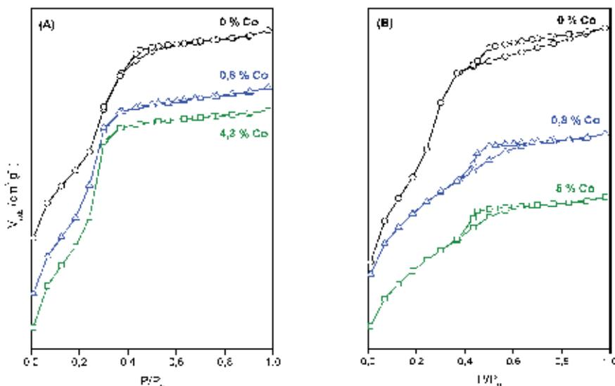
**Figure 11.** Adsorption/desorption isotherms of N<sub>2</sub> at  $-196^\circ\text{C}$  obtained for samples functionalized with Co on supports (A) MCM-41 and (B) Al-MCM-41.
