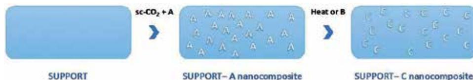
**Figure 4.** Schematic diagram for supercritical fluid deposition method. (a) Organometallic precursor, (b) reducing agent, and (c) metal nanoparticles.
