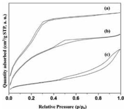
**Figure 4.** Nitrogen adsorption-desorption isotherms of (a) MCM-48, (b) TPA-MCM-48 and (c) L-arg<sub>1</sub>/TPA-MCM-48.
