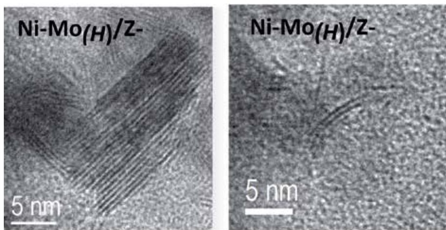
**Figure 5.** HRTEM images obtained for fresh sulfided Ni-Mo<sub>(H)</sub>/Z-1 (A) and Ni-Mo<sub>(H)</sub>/Z-2 (B) catalysts.
