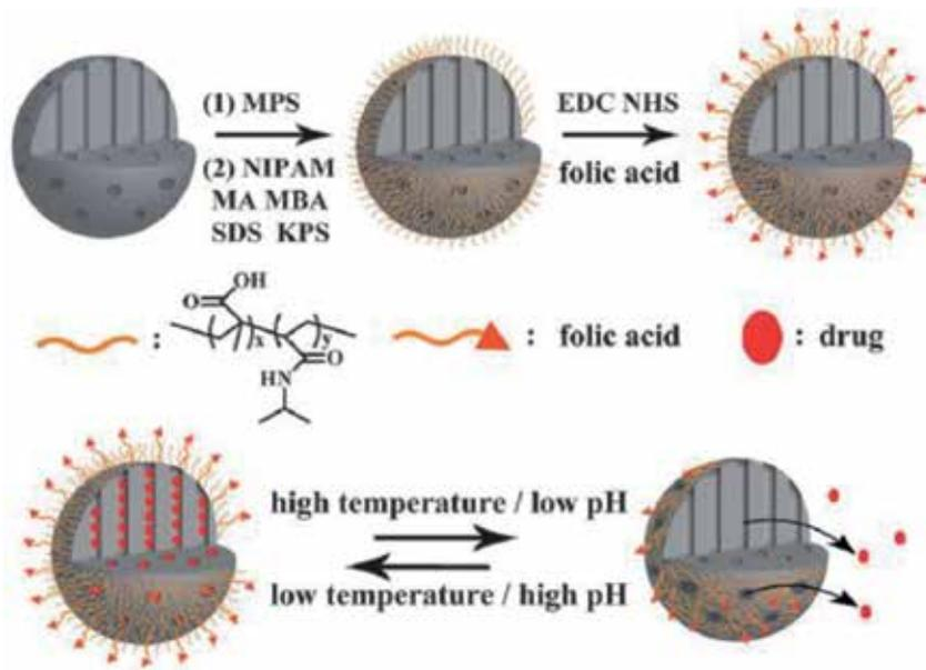
**Figure 14.** Illustration of synthesis of dual-responsive drug delivery system (reproduced with permission from Ref. [47]).
