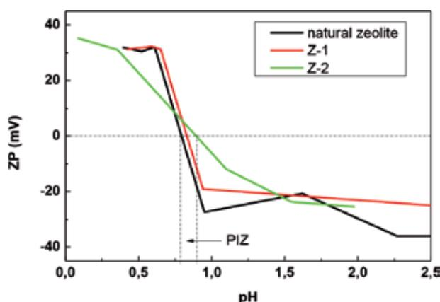
**Figure 1.** Isoelectric points (PIZ) of the clinoptilolite zeolite modified by leaching with HNO<sub>3</sub> during different times (24 and 48 h).
