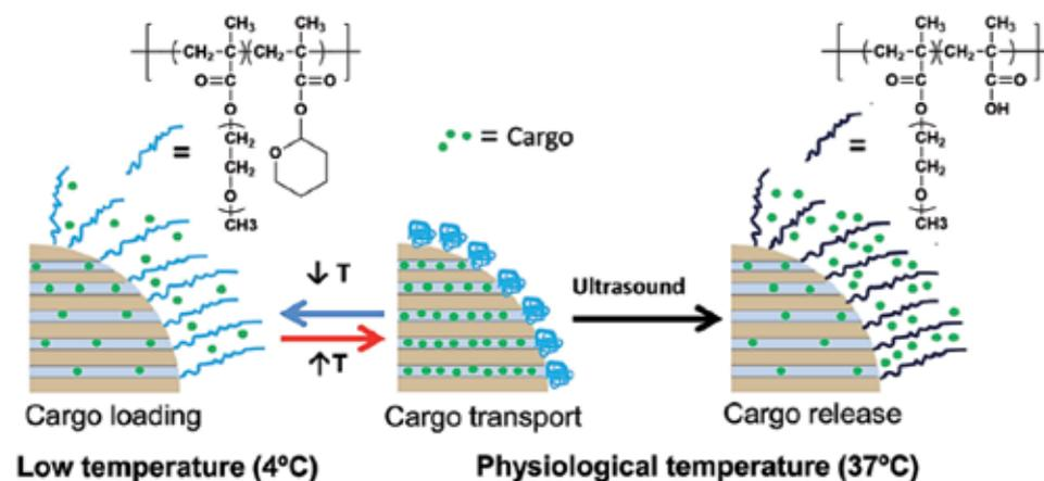
**Figure 13.** Illustration of the behavior of dual-responsive system in aqueous medium (reproduced with permission from Ref. [45]).
