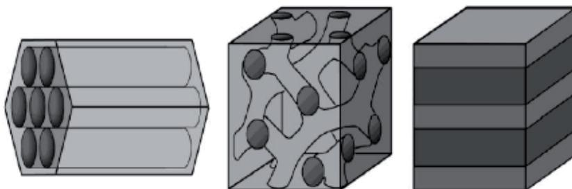
**Figure 1.** Different types of pore geometry structure for MCM family (left side for MCM-41 with hexagonal structure, center for MCM-48 with cubic structure, and right for MCM-50 with lamella structure). Reproduced with permission from Ref. [14].
