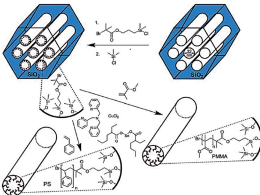
**Figure 10.** Grafting poly(methyl methacrylate) and polystyrene in the cylindrical mesopores of SBA-15 silica using ATRP (reproduced with permission from Ref. [9]).
