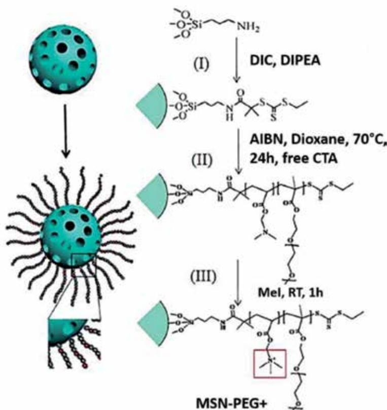
**Figure 5.** Schematic representation for synthesis of MSNs grafted with copolymer of positively charged quaternary amines and PEG via RAFT as reported by Ma et al. (reproduced with permission from Ref. [30]).
