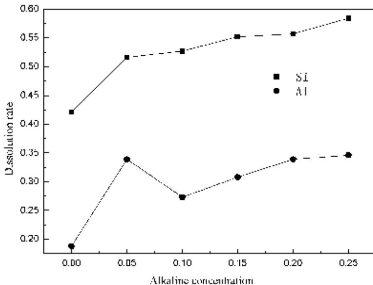
**Figure 4.** Effect of mass ratio of NaOH to solution on dissolving ratio of Si and Al 60°C, NaOH solution to clinker mass ratio of 10:1, 1 h of stirring time.
