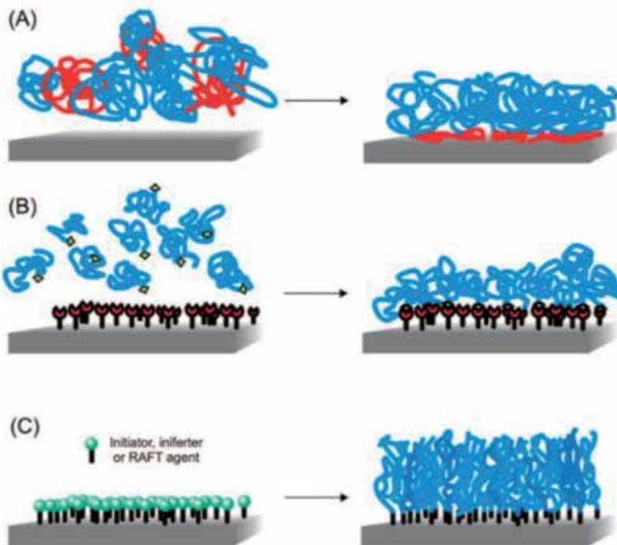
**Figure 3.** Approaches for grafting of polymer chains from solid substrate. (A) Physical adsorption, (B) Grafting-to approach, and (C) Grafting-from approach (reproduced with permission from Ref. [28]).
