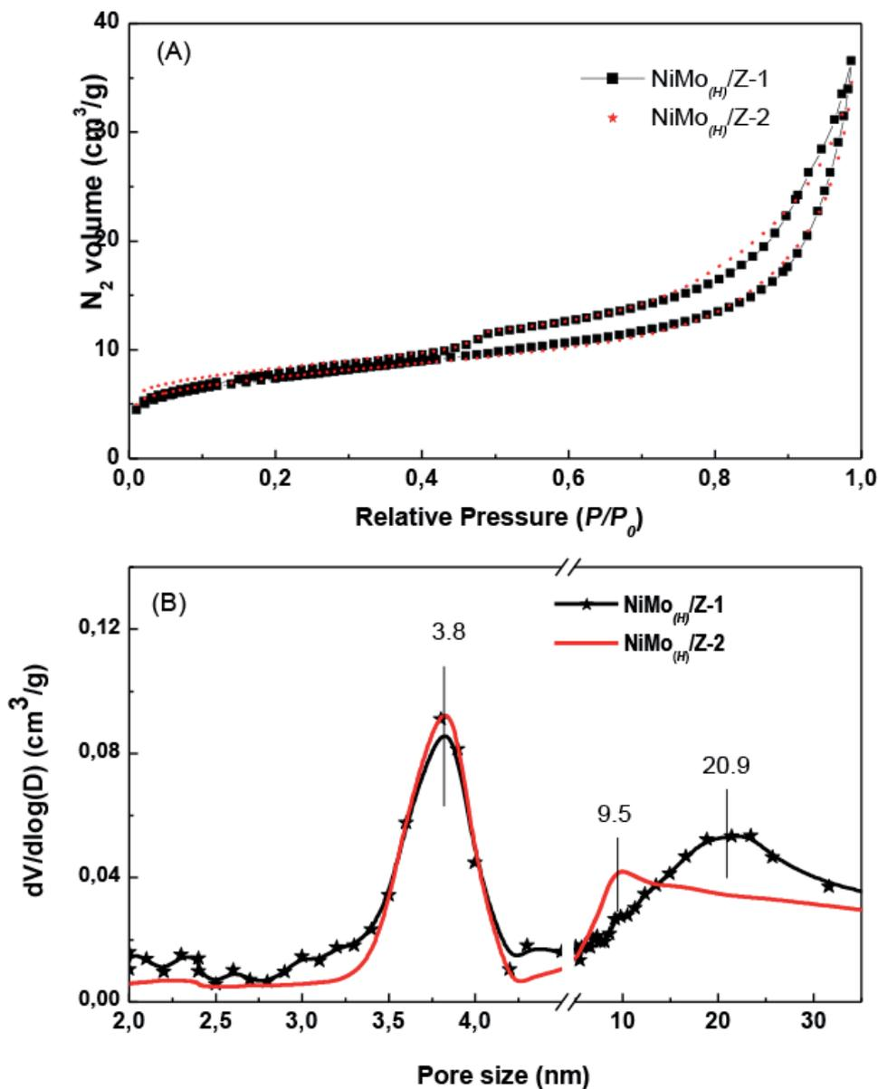
**Figure 3.**  $N_2$  adsorption-desorption isotherms of the calcined Ni-Mo<sub>(H)</sub>/Z-1(Z-2) catalysts (A) and their BJH adsorption pore size distribution (B).
