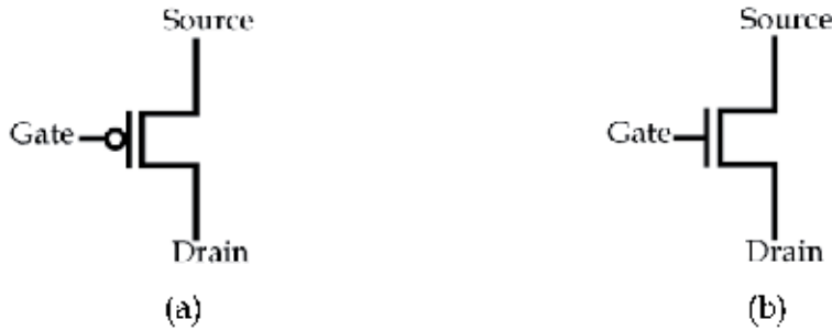
Figure 3. The symbol of (a) a PMOS transistor and (b) an NMOS transistor.
