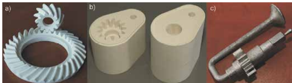
Fig. 6. Models produced by 3DP method: a) gear wheels, b) gear wheel casting mould, c) cast made in the mould from Al alloy
