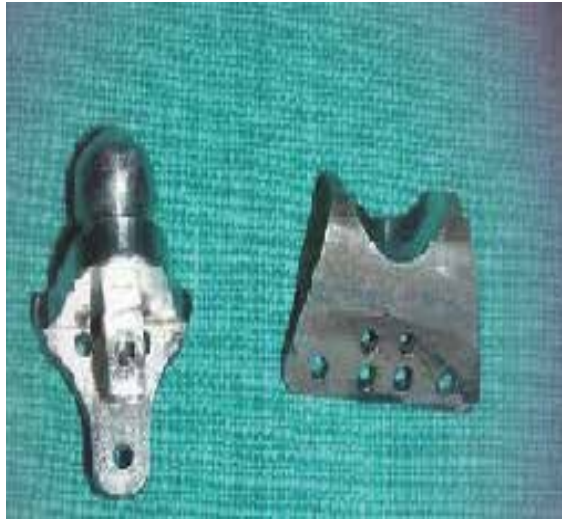
Fig. 25. Customised temporomandibular joint prepared based on RP model generated from patients CT data.
