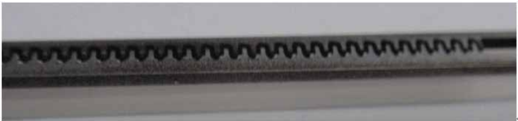
Fig. 34. Oblique teeth channel emitter obtained by assembling the wire-cutting samples and the RP sample
