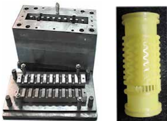
(a) The overall figure of steel mold (b) labyrinth dropper Products
