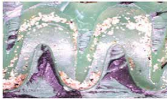
(a) starting stage of clogging
