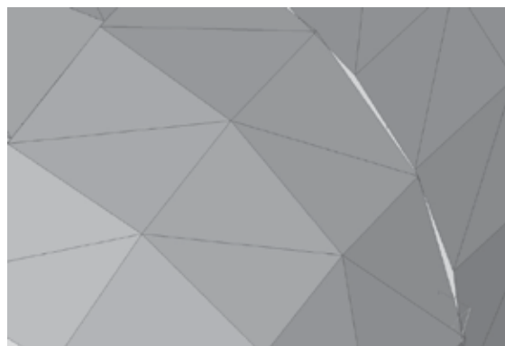
Fig. 13. Warps at the joint of surfaces in STL model
