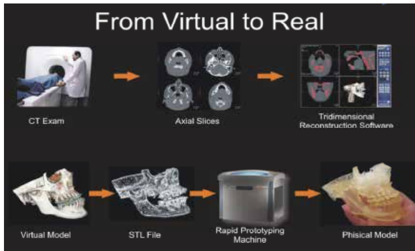
Fig. 12. Step by step sequence to fabricate a prototype of a human anatomic structure
