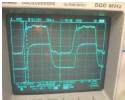
Fig. 15. Signal propagation in the WaferNet of the first test chip.
