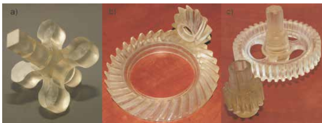
Fig. 4. Gear wheels made by SLA method: a) gear wheel of cycloidal profile, b) bevel gear wheels, c) cylindrical gear wheels
