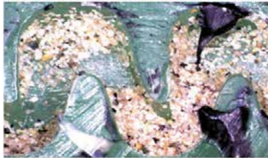
(b) developing stage of clogging
