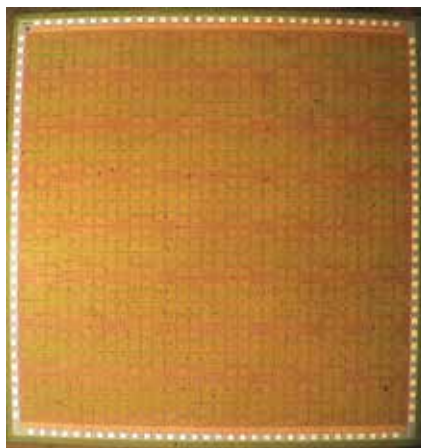
Fig. 16. Second test chip silicon die layout (Valorge, Blaquière & Savaria, 2010).
