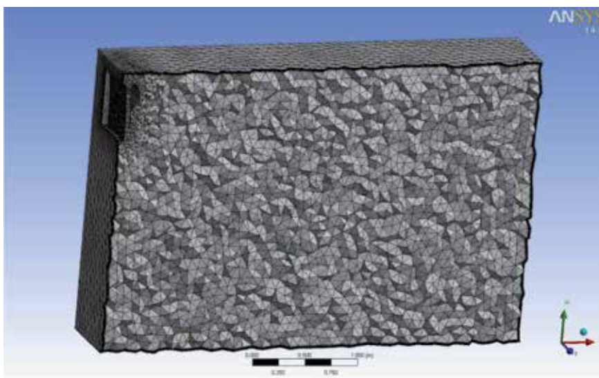
Figure 10. 3D cell grid used for medium mesh. Cross-section at the measurement plane.
