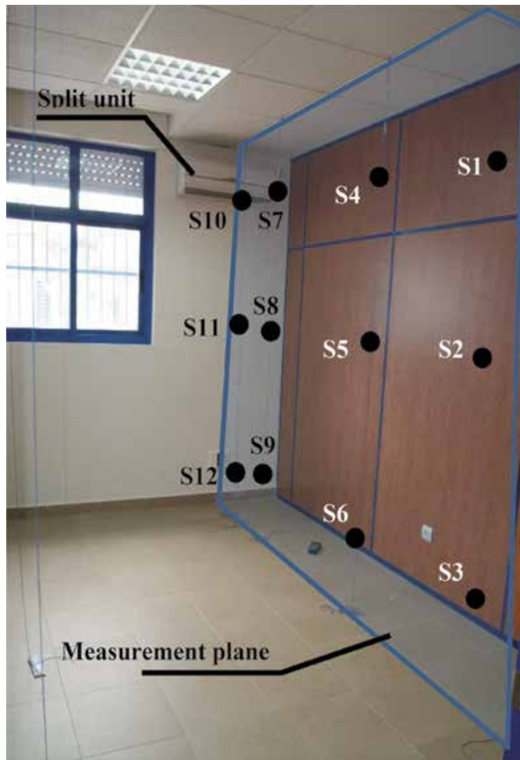
Figure 3. Location of temperature sensors in the experimental office room.
