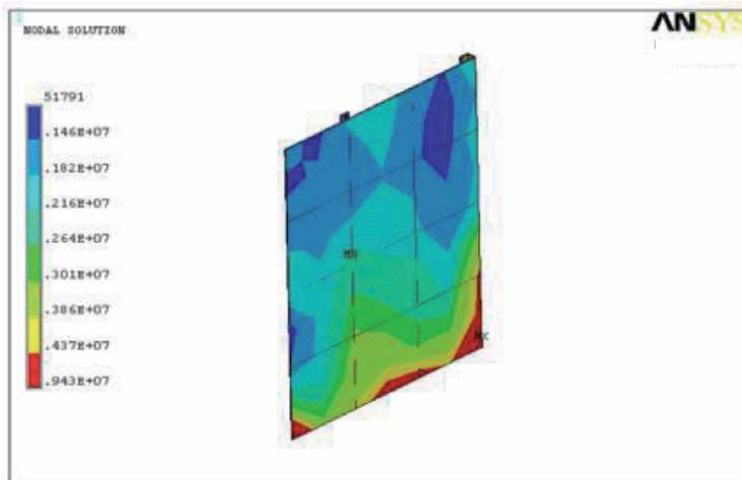
Figure 15. Distribution stress of composite ship EN AC 43100(AlSi10Mg(b)) + SiC*/15p in superstructure wall with plate thick 5 mm (max. Stress =9.43 MPa).
