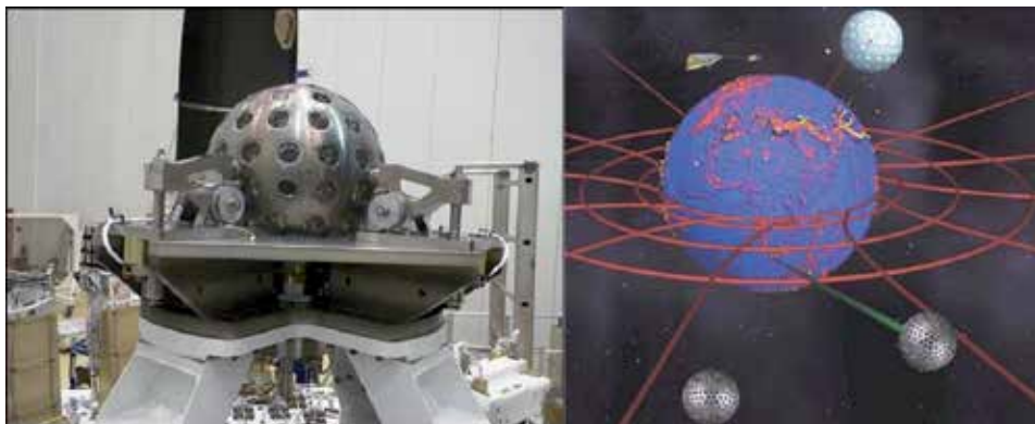
Figure 4. (Left) Image of LARES satellite (Right) Schematic view of LAGEOS-1, LAGEOS-2 and LARES in orbit for the measurement of frame dragging [8].
