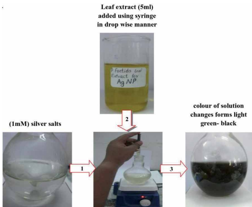
Figure 3. Complete process of green synthesis of silver nanoparticles at room temperature [18].
