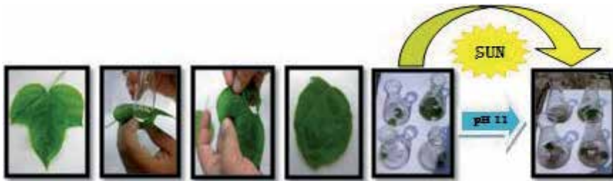
Figure 5. Leaf disc preparation using test tube for applying wound stress to P. foetida and synthesis of silver nanoparticles using leaf disc under sunlight [14].
