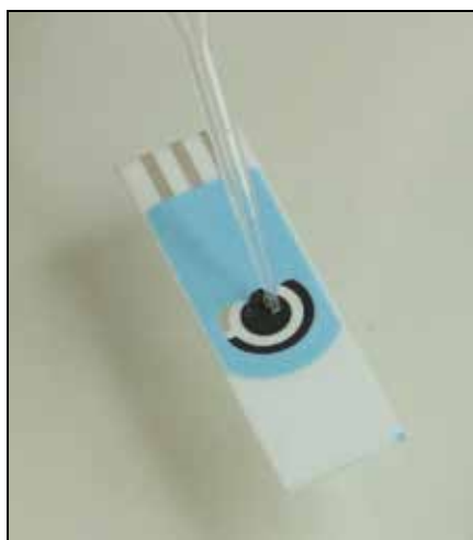
Fig. 8. Screen printed electrode used for biomediator immobilization.
