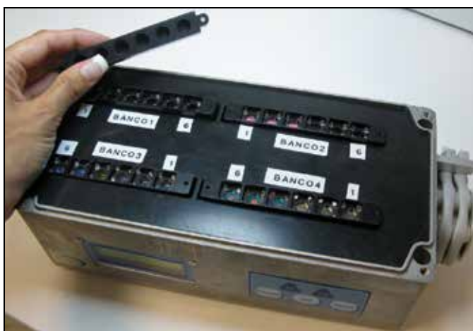
Fig. 7. Biosensing platform set-up consisting of 24 cells able to host an array of several biomediators.
