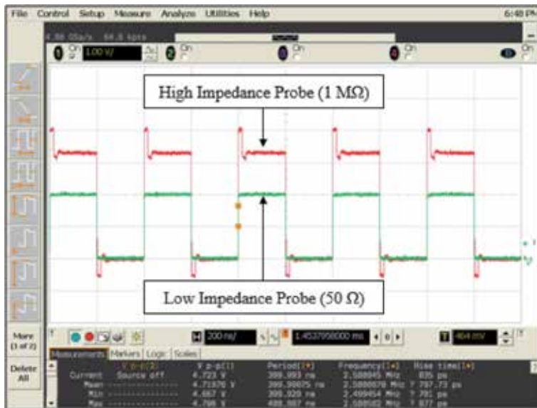
Figure 16. Clock output waveforms comparison at 2.5 MHz.
