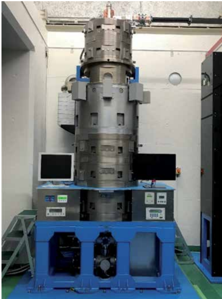
Figure 1. Photo of UEM with relativistic-energy femtosecond electron pulses constructed at Osaka University [13, 14].
