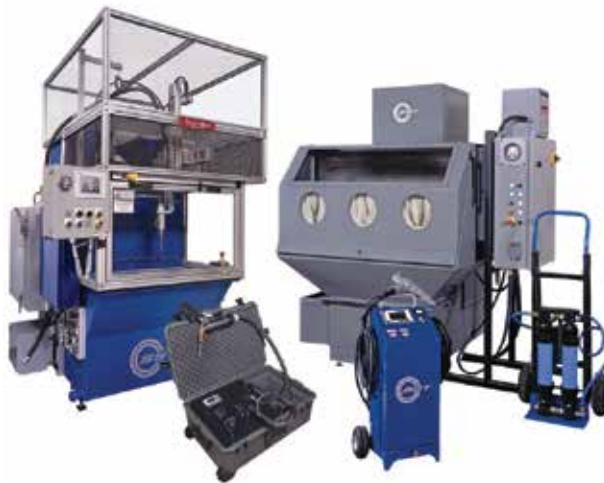
Fig. 8. Commercial low-pressure cold spray equipment (Picture courtesy of SST, a Division of CenterLine (Windsor) Ltd.).
