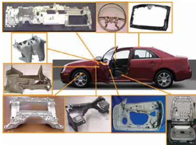
Fig. 2. Automotive applications for Magnesium alloys (Picture courtesy of Dr. Alan A. Luo, General Motors, "Magnesium Front End Development - USAMP Activities", paper presented at the SAE World Congress, Detroit, MI, April 18, 2007).
