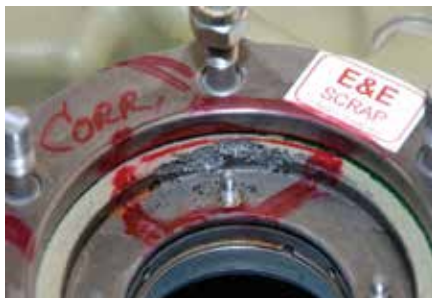
Fig. 3. Corrosion damage in magnesium alloy castings used in rotorcraft.
