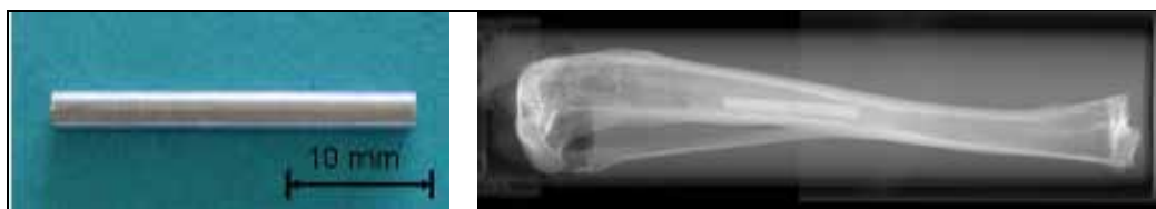
Fig. 1. Implant material and implant location: extruded magnesium pin (a) and radiographical picture of the implant location in the rabbit tibia (b)
