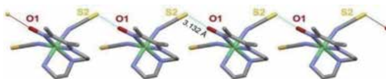
Figure 13. S\cdots O interaction in the crystal of complex 1 (hydrogen atoms are omitted for clarity).
