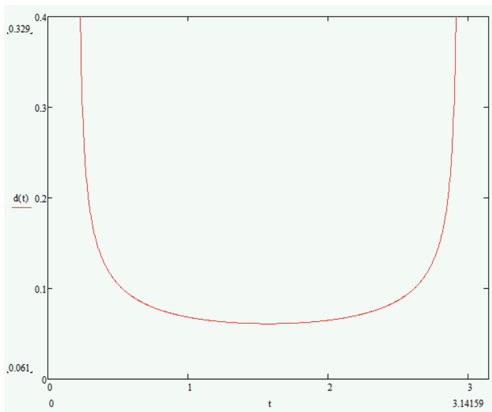
Fig. 5. Duty cycle changes in response to varying input voltage in discharging mode.
