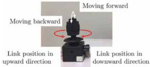
Figure 5. Joystick for manipulating Robot A .
