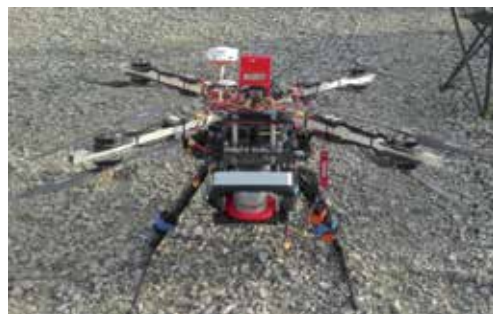
Figure 1. One of the UAV used for the development of perception tasks in the AEROARMS project. Several sensors were deployed, processing them with a set of SBCs (single-board computers), including a Velodyne LiDAR, two different cameras, ultrasonic range-finder (height), and optical flow.
